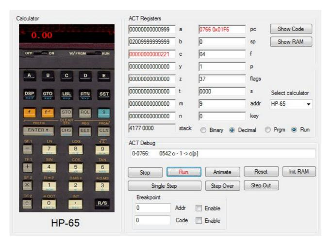
The HP-65 was the first programmable HP calculator. It uses an instruction set, which is related to the Classic ACT processor, but uses special pointer instructions for handling the program memory. Have fun to see how immensely complicated the firmware does its job. Of course there is no Card Reader functionality possible with this virtual calculator.
